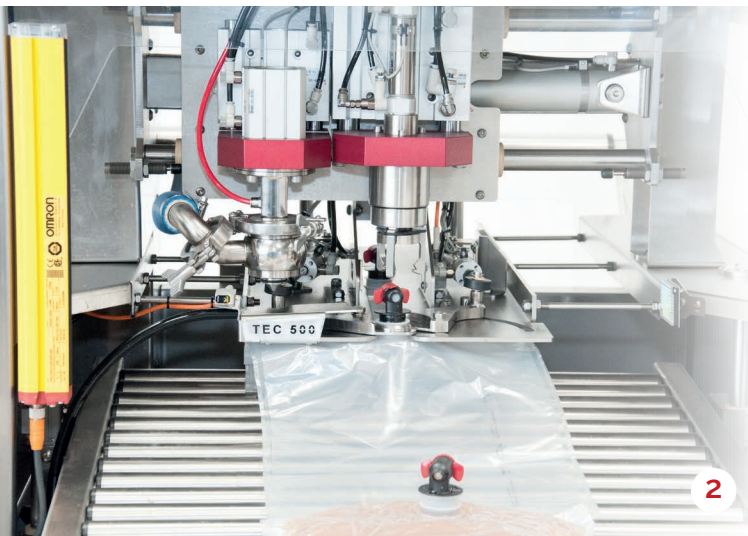
Caption: 1) Service window with compressed air maintenance unit, 2) Filling unit of individual and endless pouches, 3) Feeding roll for endless pouches
