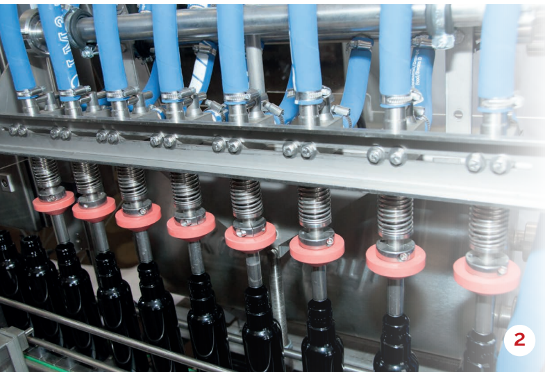
Caption: 1) Ultrasound sensor for bottle count , 2) Filling unit with adjustable valves, 3) Sorting table with transition to capping strap
